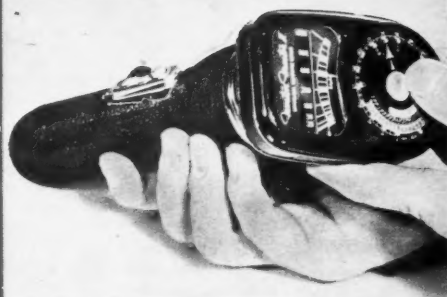
By checking your meter against the same flashlight (always equipped with fresh batteries) you can readily determine if it is still up to par. Test in contact with lens.
